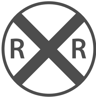
Figure 2.17 Round Yellow Warning Sign
